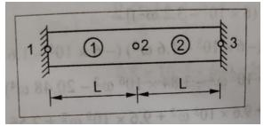
4. (a) An aluminium alloy fin of 7mm thick and 50mm long protrudes CO5 - App (20) form a wall, which is maintained at 120°C. The ambient air temperature is 22°C. The heat transfer coefficient and thermal conductivity of the fin material are 140W/m<sup>2</sup>K and 55W/mK respectively. Evaluate the temperature distribution of fin.
