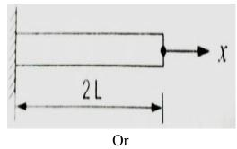
(b) Compare the natural frequency of vibration for a beam fixed at CO4 - Ana (20) both ends. The beam has mass density ρ, modulus of elasticity E, cross sectional area A, moment of inertia I, and length 2L. The beam is discretized into two elements of length L.
