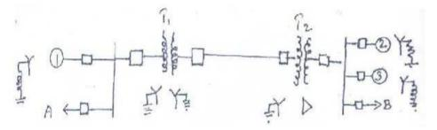
Generator No. 1: 30 MVA, 10.5 kV, X'' = 1.6 Ohm Generator No. 2: 15 MVA, 6.6 kV, X'' = 1.2 Ohm Generator No. 3: 25 MVA, 6.6 kV, X'' = 0.56 Ohm T1 (3phase): 15 MVA, 33/11 kV, X = 15.2 Ohm per phase on HT side T2 (3phase): 15 MVA, 33/6.2 kV, X = 16 Ohm per phase on HT side Transmission line: 20.5 Ohm/phase Load A: 15 MW, 11kV, 0.9 P.F. lagging Load B: 6.2KV, 34 MW+j20.07 MVAR.
