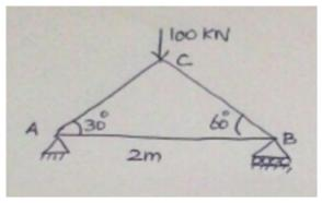
17. (a) Determine the bending moments for structure as shown in figure by CO4-Ana (16) slope deflection method. Sketch the super imposed bending moment diagram.
