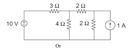
(b) Find the Thevenin's and Norton's equivalents for the circuit shown CO2-App (16) in Fig. with respect to terminals ab.
