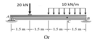
(b) A beam AB of span 3m, overhanging on both sides is loaded as CO2 App (16) shown in Fig. Determine the reactions at the supports A and B.
