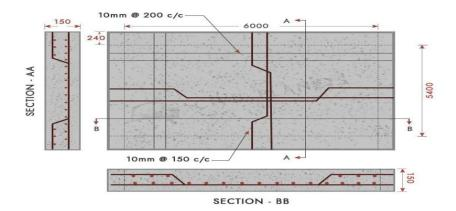
From the Drawing Slab Size = 6000 x 5400 x 150 mm 10 mm dia Main Bars @ 150 mm c/c along shorter direction 10 mm dia Main Bars @ 200 mm c/c along longer direction Development Length Ld = 40d
