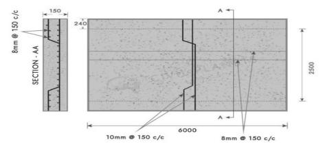
From the Drawing - Slab Size = 6000 x 2500 x 150 mm
