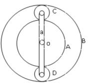
20. (a) A belt drive transmits 8 kW of power from a shaft rotating at 240 rpm to another shaft rotating at 160 rpm. The belt is 8mm thick. The diameter of the smaller pulley is 600 mm and two shafts are 5 m apart. The coefficient of friction is 0.25. If the maximum stress in the belt is limited to 3 N/mm<sup>2</sup>, find the width of the belt for (i) an open belt drive and (ii) a cross belt drive. (16)
