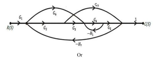
(b) (i) Obtain the closed loop transfer function C(s)/R(s) of the system whose block diagram is shown in figure. (16)
