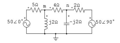
12. (a) Find Thevenin's equivalent circuit for the circuit shown below. (16)
