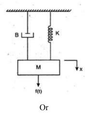
(b) Draw the signal flow graph and find C(S) / R(S) using Mason's gain formula for the system shown in figure. (16)
