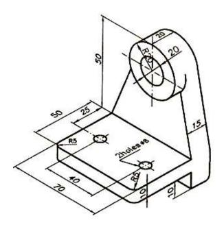
(b) Draw the orthographic view (Plan, Elevation and side view) for the given figure. All Dimensions are in mm. (20)
