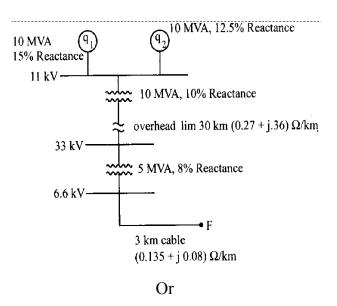
(b) A symmetrical fault occurs at bus 4 for the system shown below. CO3-App (16) Determine the fault current and post fault voltages using Z bus building algorithm.
