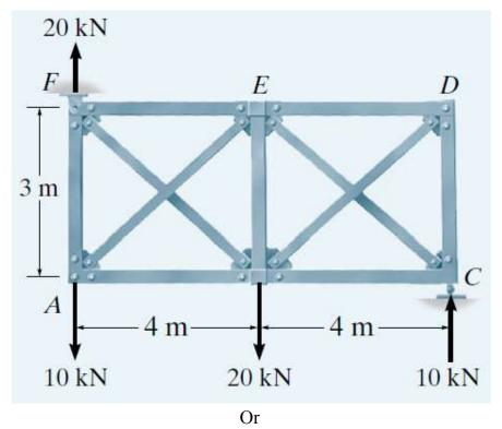
(b) Cross bracing is used to provide lateral support for this bridge CO5-Ana deck due to the wind and unbalanced traffic loads. Analyse (approximately) the forces in the members of this truss. Assume the diagonals are slender and therefore will not support a compressive force. The loads and support reactions are shown in Fig.
