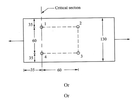
(b) A tension member consists of two angle section and carries a load of 200kN. Design the member when both the angles are connected (i) On both sides of Gusset plate (ii) On the same side of Gusset plate.
