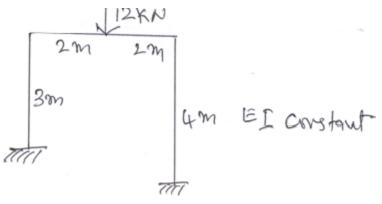
13. (a) Analyse the portal frame shown in fig by moment distribution CO3- Ana (16) method.
