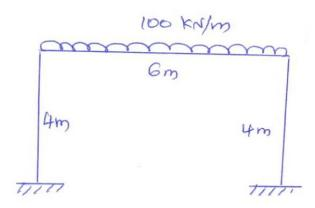
13. (a) Analyze the frame shown in figure By moment distribution method and draw the SFD and BMD. (16)
