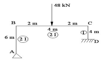
14. (a) Apply the continuous beam ABCD shown in figure by Flexibility matrix method. Take EI=Constant. Also sketch the shear force and Bending Moment diagram. (16)
