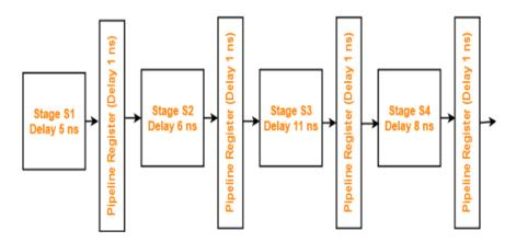
What is the approximate speed up of the pipeline in steady state under ideal conditions when compared to the corresponding non-pipeline implementation?
