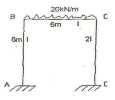
19. Apply the continuous beam ABCD shown in figure by Flexibility matrix method. Take EI=Constant. Also sketch the shear force and Bending Moment diagram. (10)
