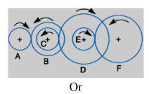
(b) In a reverted epicyclic gear train, the arm A carries two gears B CO3- App and C and a Compound gear D - E. The gear B meshes with gear E and the gear C meshes with gear D. The number of teeth on gears B, C and D are 75, 30 and 90 respectively. Find the speed and direction of gear C when gear B i s fixed and the arm A makes 100 r.p.m. clockwise.
