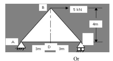
(b) Determine the horizontal displacement at support D of the frame CO2-Ana (16) shown in Fig. Take I =  $300 \times 10^{-6} \text{ m}^4$  and E =  $200 \times 10^6 \text{ kN/m}^2$ . Use Principle of Virtual work.
