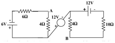
(ii) Determine the power dissipation in the  $4\Omega$  resistor of the given CO1-U (8) circuit shown in fig. using mesh/nodal analysis.
