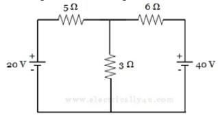
(ii) Determine the current I using network reduction technique. CO1-U (8)
