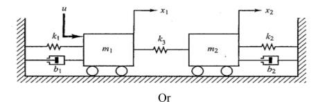
(b) Determine the transfer function  $X_2(S)/F(S)$  of the mechanical CO2- App (16) system shown in Fig.
