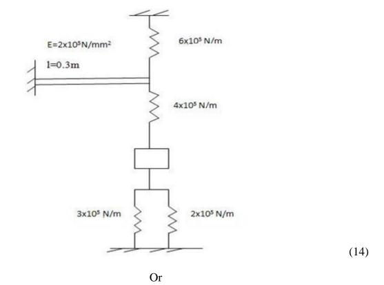
(b) Formulate the equation of motion and find the natural frequency for the following system.
