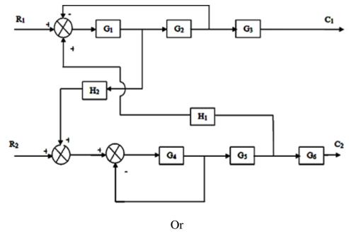
(b) Using block diagram reduction rules, convert the block diagram to a simple loop. (16)
