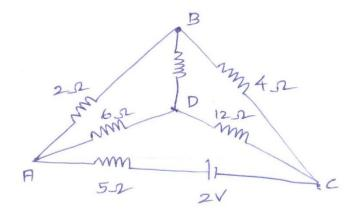
17. (a) Find the value of *RL* in the circuits given for maximum power transfer to it.Find maximum power. (16)
