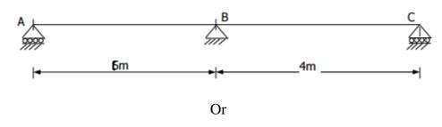
(b) Using Muller Breslau Principle, compute the influence line ordinates for every 2m interval (i) Reaction at B and (ii) Moment at A for the propped cantilever shown in below figure. (16)
