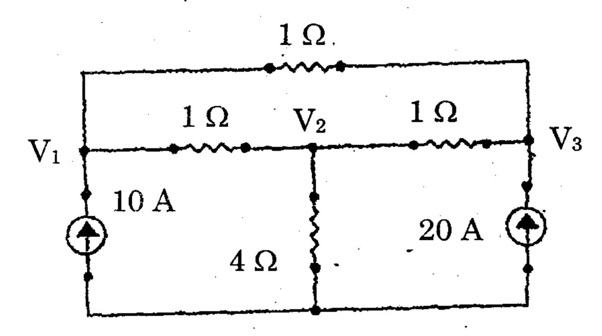
(ii) Solve for  $I_1, I_2$  and  $I_3$ , in the circuit shown below, by mesh current method. (8)
