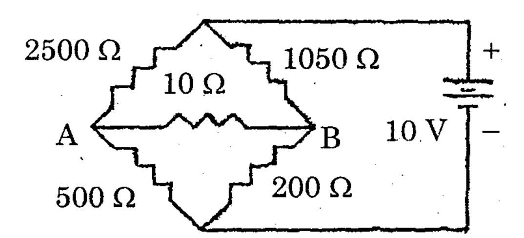
(ii) Obtain the Norton's equivalent circuit for the network shown below and find the current through AB. (8)
