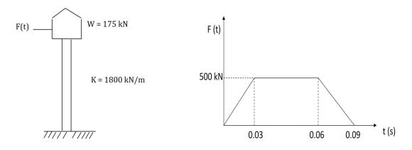
12. (a) Determine the natural frequencies and mode shapes for the framed structure shown in figure. The floor may be considered as rigid. (16)
