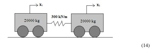
13. (a) Calculate the natural frequency and corresponding mode shapes for the system as shown in the figure. Also verify the orthogonal conditions.
