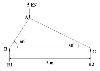
(b) A truss of 12 m span is loaded as shown in figure. Find the forces in the members of the truss by method of sections. (16)
