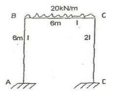
(b) Analyse the portal frame shown in Figure by using moment distribution method and draw BMD. (16)
