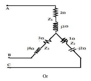
(b) (i) State the Thevenin's theorem and find the current through branch a-b of the network shown in below figure. (10)
