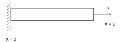
13. (a) Consider a bar as shown in below figure and having  $A = 750mm^2$ ,  $E = 2 \times 10^5 mm^2$ . If  $\mu_1 = 0.5mm$  and  $\mu_2 = 0.625mm$ . Calculate the following (i) Displacement at point, *P* (ii) Strain (iii) Stress (iv) Element stiffness matrix (v) Strain energy *u*. (16)
