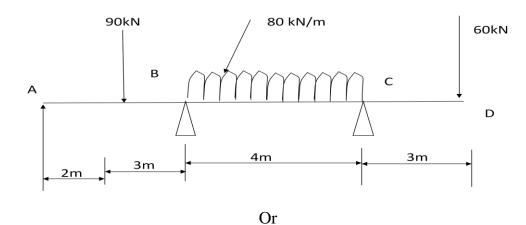
(b) Analysis the frame as shown in figure using moment distribution method and draw BMD. (16)
