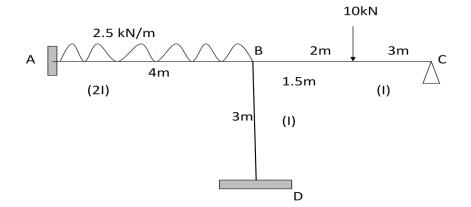
13. (a) Draw BMD for continuous beam as shown in below figure, if the support *B* sinks by 2.5*mm*. Take  $I=3.5\times10^7 \text{ mm}^4$ ,  $E=200 \text{ KN/mm}^2$  Using moment distribution method.
