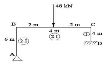
14. (a) Using flexibility matrix method analyzes the given beam and draw the BMD. (16)
