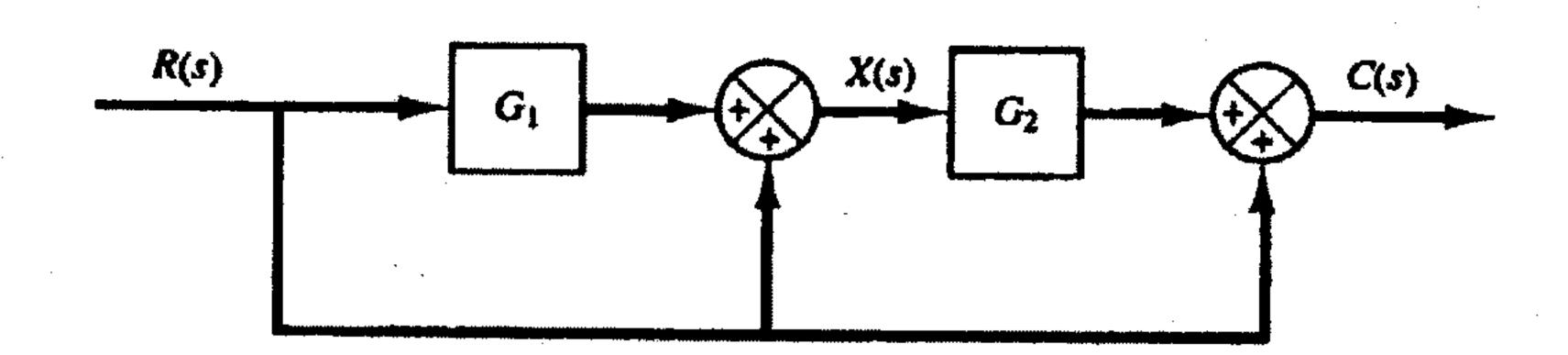
3. Find the settling time and Peak time for the given block diagram.
