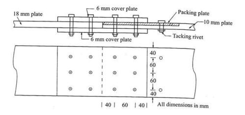
17. (a) Design a channel section to carry an axial tension of 300kN. Take  $f_y = 250$  N/mm<sup>2</sup>. Also design the riveted joint at the end. (16)
