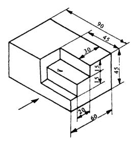
(b) Draw the plan view, front view and side view of the following figure. (20)
