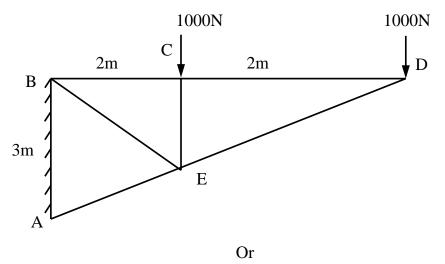
(b) Determine the forces in all members of a truss as shown in below figure. (16)
