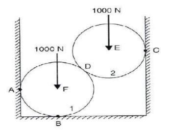
12. Solve the resultant in magnitude and direction and also locate its points CO2- App (8)of application and edge of intersection.
