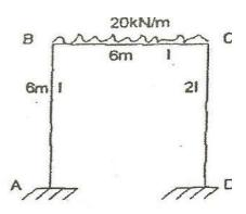
14. Apply the continuous beam ABCD shown in figure by Flexibility matrix method.Take EI=Constant. Also sketch the shear force and Bending Moment diagram. (8)
