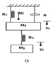
(b) Write the differential equations governing the mechanical system shown in Fig. 3. Draw the force-voltage and force-current electrical analogous circuits and verify by writing mesh and node equations. (16)
