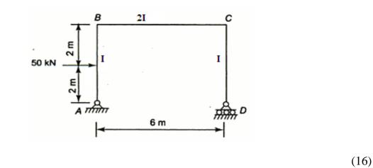
12. (a) Analyze the beam shown in below figure by slope deflection method and draw the bending moment diagram.
