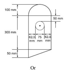
(b) Find the moment of inertia of the section shown in figure, about the centroidal axes.(Dimensions in mm). (16)
