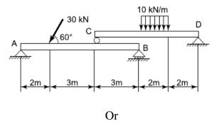
(b) Find the pin reaction at *A* and the knife-edge reaction at *B*.
