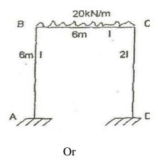
(b) Analysis the frame as shown in figure using moment distribution method and draw BMD. (16)
