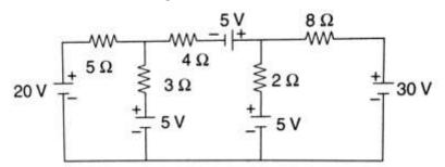
(a) (ii) Determine the total equivalent resistance for the circuit
