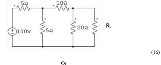
(b) For the circuit shown below, determine Thevenin's equivalent circuit. (16)
